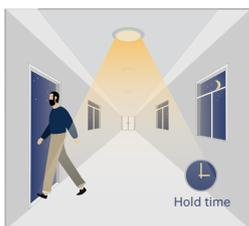
After motion is no longer detected, fixture remains at 100% for hold time.
