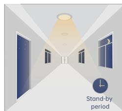
After pre-set hold time period it will dim light to standby dimming level again and always keep it.
